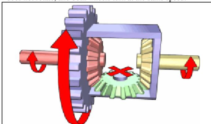
Figure 1 : Differential Dynamics When Vehicle Runs on Straight Path.
