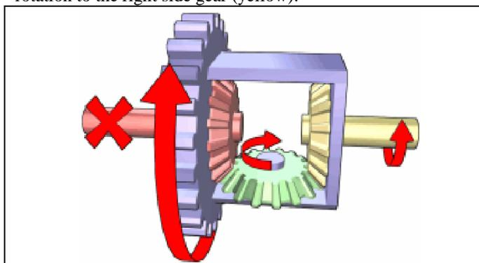
Figure 2 : Differential Dynamics When Vehicle Takes Turn.
