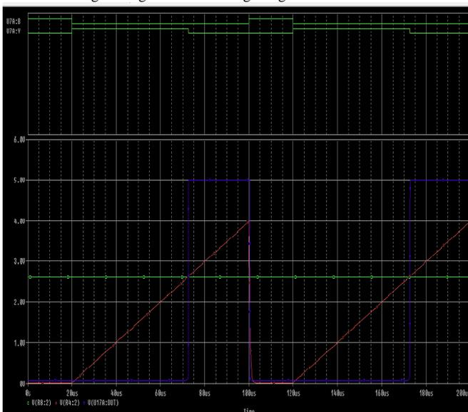
Fig.7: Output Waveform of SMPS using Integrator circuit
