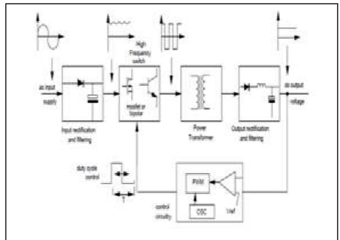
Fig.1: Basic Switch Mode Power Supply Block Diagram
