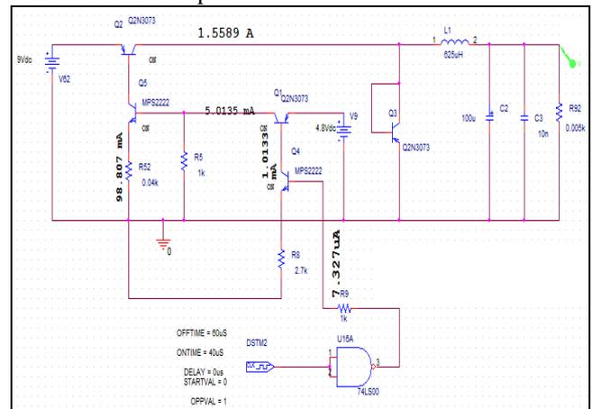
Fig.4 Switch Drive Circuit
