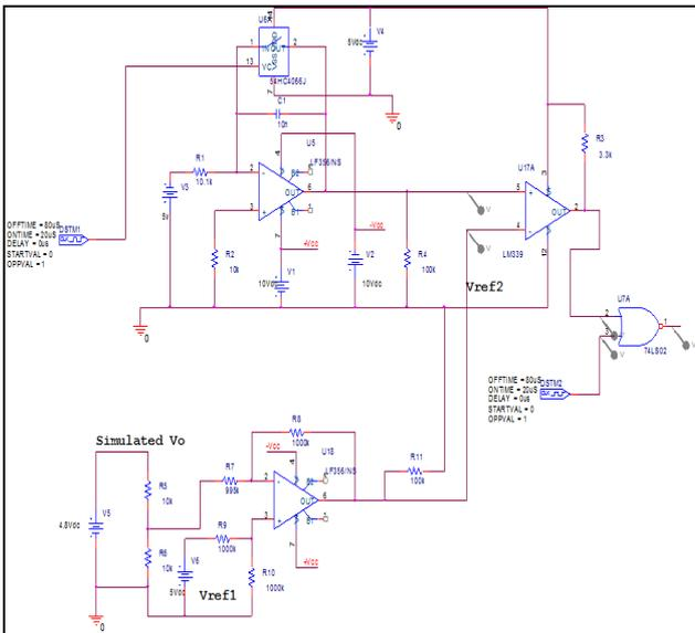
Fig6:Design of SMPS using Integrator circuit
