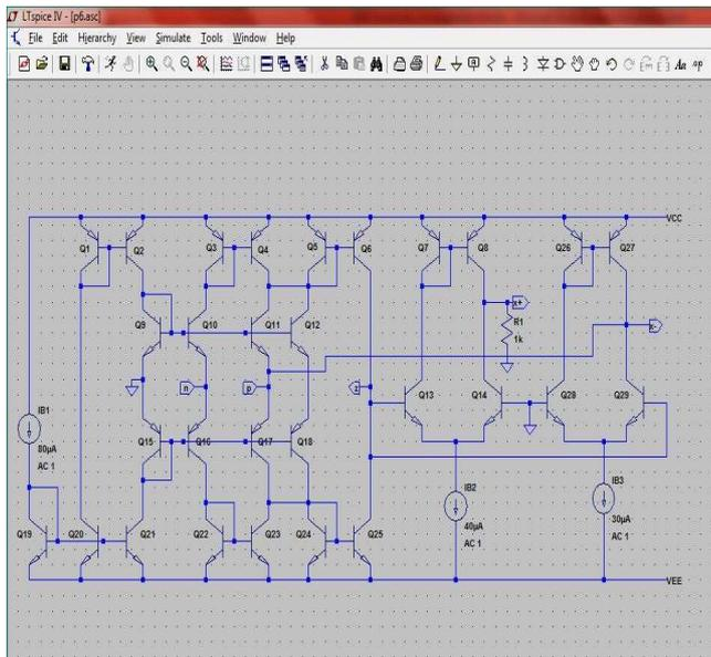
Fig.4 MO-CCCDTA based Schmitt trigger on LT spice
