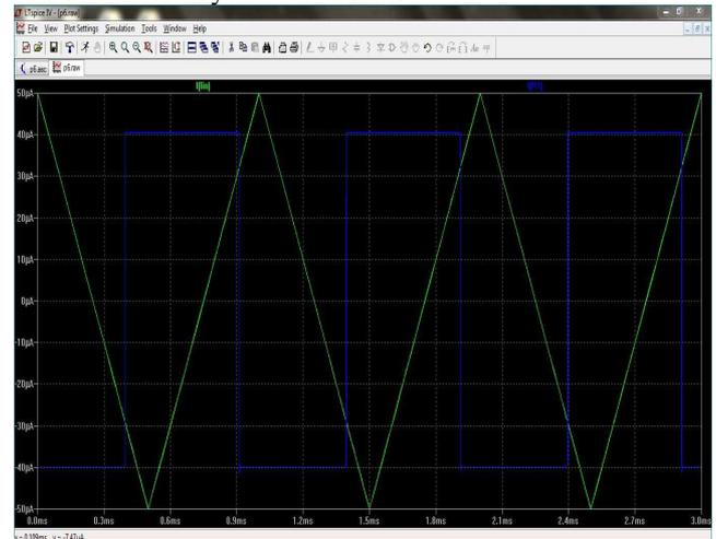
Fig.5 LT spice waveform of non-inverting MO-CCCDTA based Schmitt trigger
