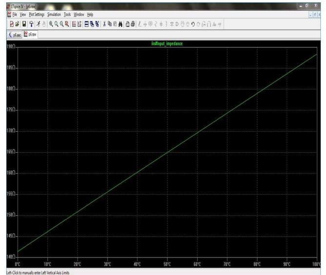
Fig.10 Variation in Input Impedance
