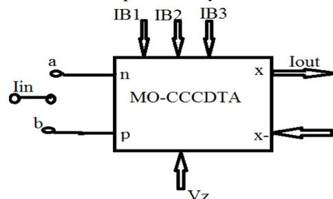
Fig.1 MO-CCCDTA block diagram
