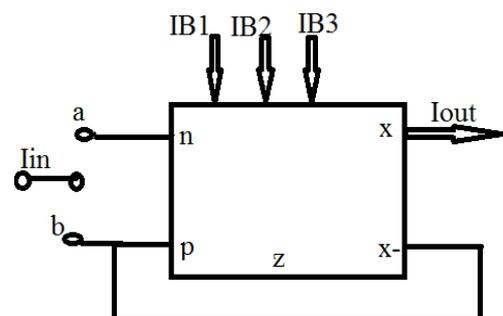
Fig.3 MO-CCCDTA based Schmitt trigger
