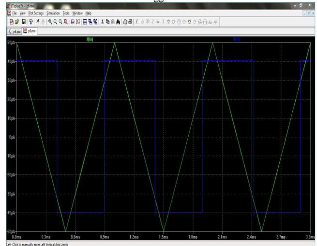
Fig.6 LT spice waveform of inverting MO-CCCDTA based Schmitt trigger
